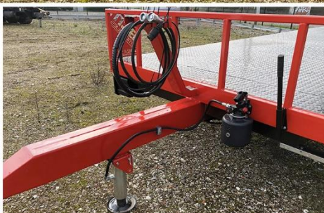
Surface utile : 7m00 x 2m54, Tandem susp. lame de ressorts, RC 235/75 R17.5, Pompe à main Sarl BCM - D910 La Normandie - 37110 VILLEDOMER - 02.47.550.100 - www.remorques-bcm.com
