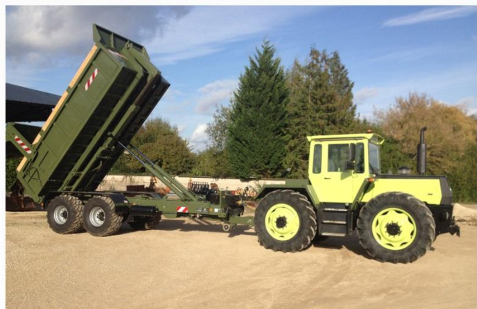
Bras reconditionné, Freinage AIR 40km/h, RC 560/60 R22.5, Pompe engrenages 118l/min, attelage Calotte
